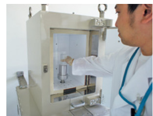
A germanium detector, which makes it possible to measure radioactive cesium precisely
