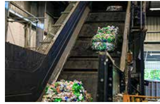
Recycling bales entering production process at Unifi warehouse - PBV partners with Unifi for the processing of recycling materials
