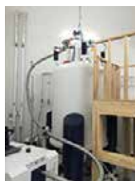
800 MHz superconducting nuclear magnetic resonance equipment
